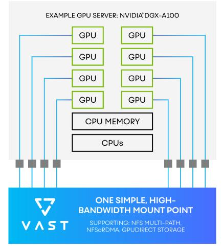
Most enterprise storage systems adhere to the standard NFS/TCP model that has been the core offering of scale-out NAS providers for decades. New AI machines need more than the 2GB/s of read throughput that a standard TCP NFS client can provide. This single-stream, non-RDMA limitation is why organizations abandon NFS in favor of parallel file systems and chose performance over simplicity.
